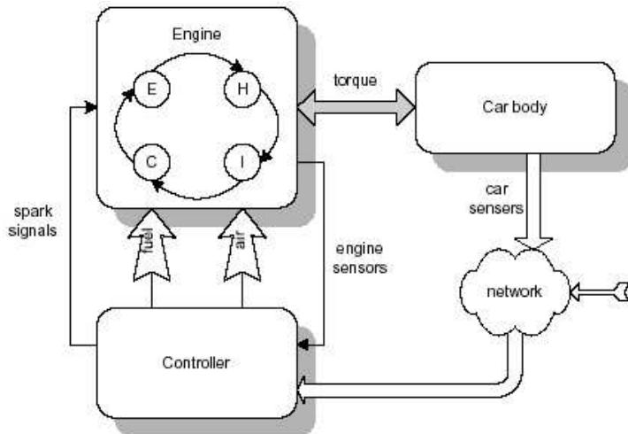
A cylinder of an internal combustion engine has four working phases: intake, compress, explode, and exhaust. The engine generates torque that drives the power train and the car body.
